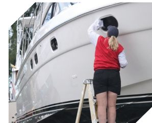
Applying Glidecoat Surface Wipe (de-contaminate) before coating. Surfaces have been compounded and polished.
