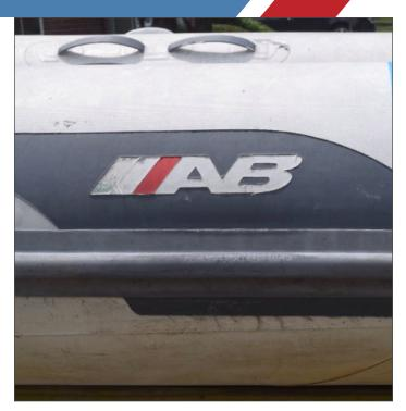
This is an all-too-common look for inflatables faded from sun, covered in dirt because of the difficulty keeping clean and damaged from years of use.
